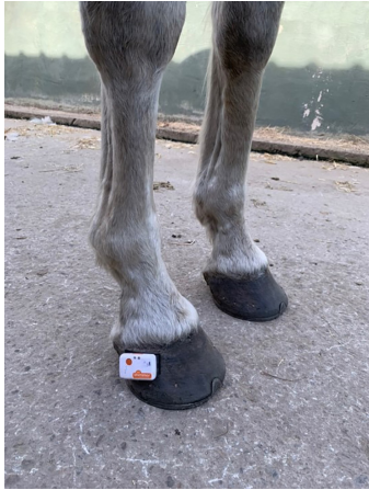
Figure 1: Shimmer IMU attached to the lateral aspect of the hoof wall using sticky-back hook-and-loop fastenings.
