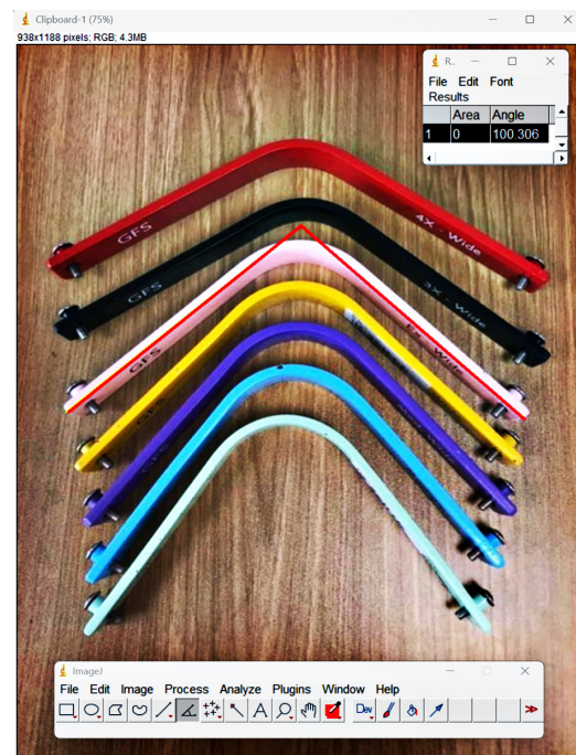
Figure 5: Measurement of the angle (red line) of the GFS Monarch Extra-Wide gullet bar (pink) using ImageJ, indicating an angle of 100.3°.
