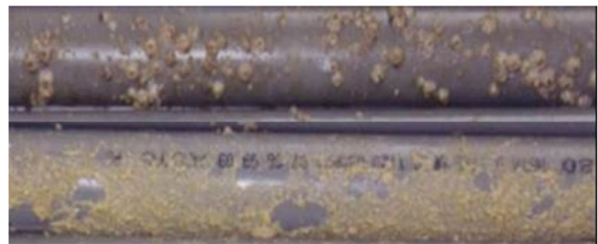
Figure 4: Two biofilm slide tube holders: above from open sea (location S3, Figure 1) and below from brine discharge channel (location S1, Figure 1). Note shells in the open sea and lack thereof in the brine discharge channel.
