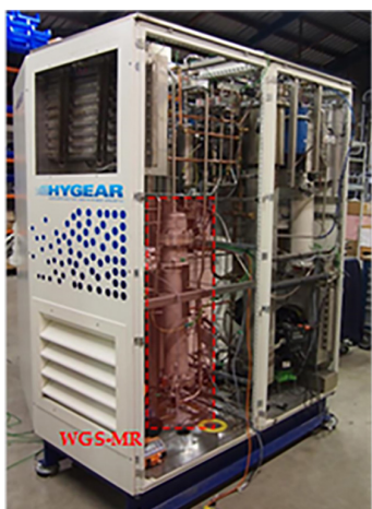
Figure 7: Picture of the prototype reactor for the WGS process where the placement of the WGS-MR is highlighted. Reprinted from [118].
